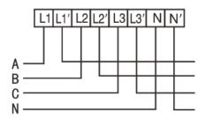
(2) three phase four wire through current transformer connection
