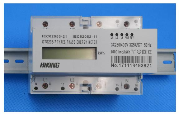
The meter is used in three phase four wire/three phase three wire/two phase three wire power grid. The meter is designed to measure AC active energy. All of its functions comply with the relative technical requirement for class 1 three phase watt hour meter in IEC62053-21. It is a long life meter with the advantage of high stability, high over load capability, low power loss and small volume.
